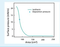
CdSe-NANOCRYSTALS WERE COMPRESSED TO A SURFACE PRES-SURE OF 12 mN/m FOR DEPOSITION. The figure above displays the surface pressure - area isotherm obtained during compression. Adapted with permission from Langmuir 2010, 26 (11), pp 7732-7736. Copyright 2010 American Chemical Society.
